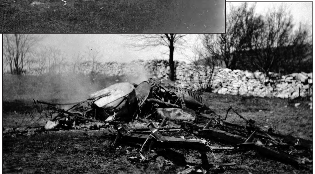
Above and Right: Sometimes the planes never left the field. As this plane was preparing to depart the Bellefonte Air Mail Field on November 14, 1919, its Liberty engine caught fire and the wooden plane was quickly destroyed.
